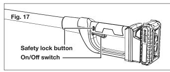
3. To turn the tool OFF, release the On/Off switch (Fig. 17).
