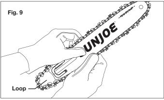
6. Hold the chain in position on the bar and place the loop around the sprocket. Fit the bar flush against the mounting surface so that the bar stud hole are aligned with the long slot of the bar (Fig. 10).
