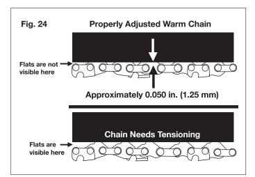
**NOTE:** A new chain tends to stretch. Check the chain tension frequently and re-tension as needed.
