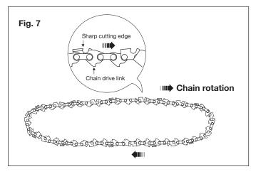
5. Starting at the tip, mount the chain drive links into the bar groove, leaving a loop at the back of the bar. The chain will loosely fit until it is placed on the sprocket (Figs. 8 – 9).
